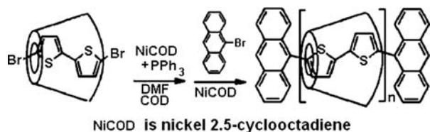
Scheme 7. Preparation of oligothiophene/ \beta -CD rotaxanes with anthryl groups as the end stopper (46).
